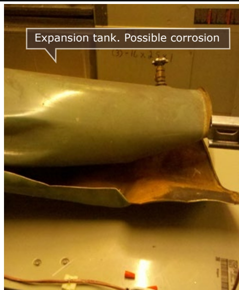
Air tank. Failed due to corrosion.
